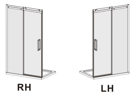
The slider is ok to be installed in left hand and right hand. The following step is based on right hand. For left hand, please follow the step in mirror direction.
